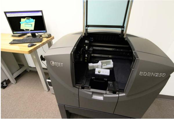
3-D printing is an additive process for converting digital 3-D models of objects into physical 3-D objects themselves. In an additive process, a modeled object is created by laying down successive layers of material until the entire physical object is created. Each of these layers is essentially a thinly sliced horizontal cross section of the eventual object.
