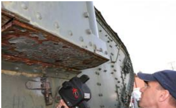
Figure 13. K-Scan Measurement of Sponson Bottom
