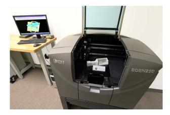
3-D printing is an additive process for converting digital 3-D models of objects into physical 3-D objects themselves. In an additive process, a modeled object is
